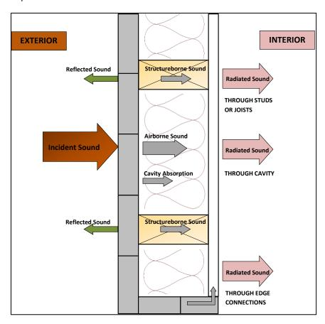
Figure B-15 Depiction of Sound Transmission through Built Construction
