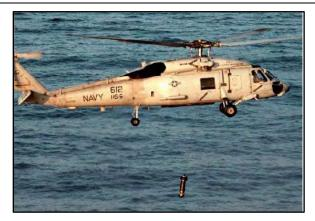
Figure A-6: Helicopter Dipping Sonar
