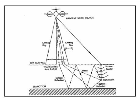
Figure B-9 Characteristics of Sound Transmission Through the Air-Water Interface
