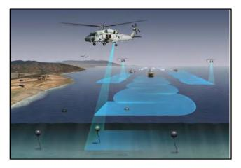
Figure A-1: Airborne Laser Mine Detection System
