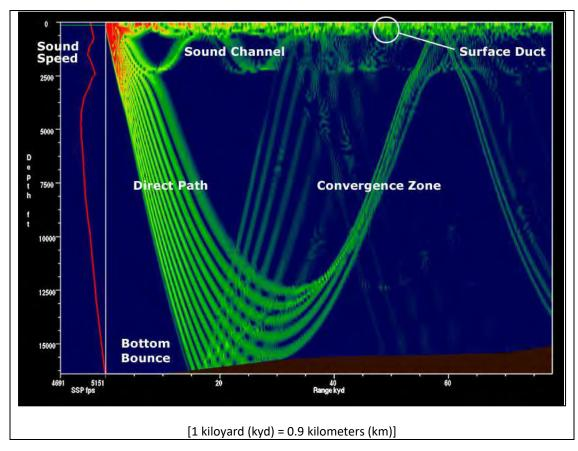
Figure B-8 Sound Propagation Showing Multipath Propagation and Conditions for Surface Duct
