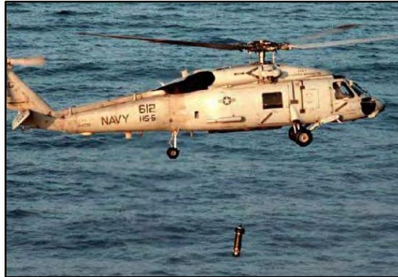
**Figure A-6: Helicopter Dipping Sonar**
